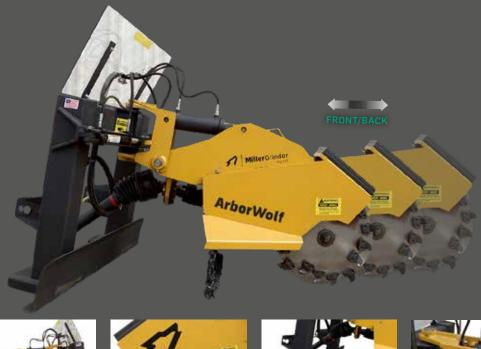
(X-Y-Z) hydraulic positioning of the cutting blade: up/down, tele in/ tele out & swing left/swing right. Allows operator to anchor the grinder firmly on its backfill blade, hydraulically move the cutter and grind an average 36"stump without having to reposition the machine, greatly increasing
